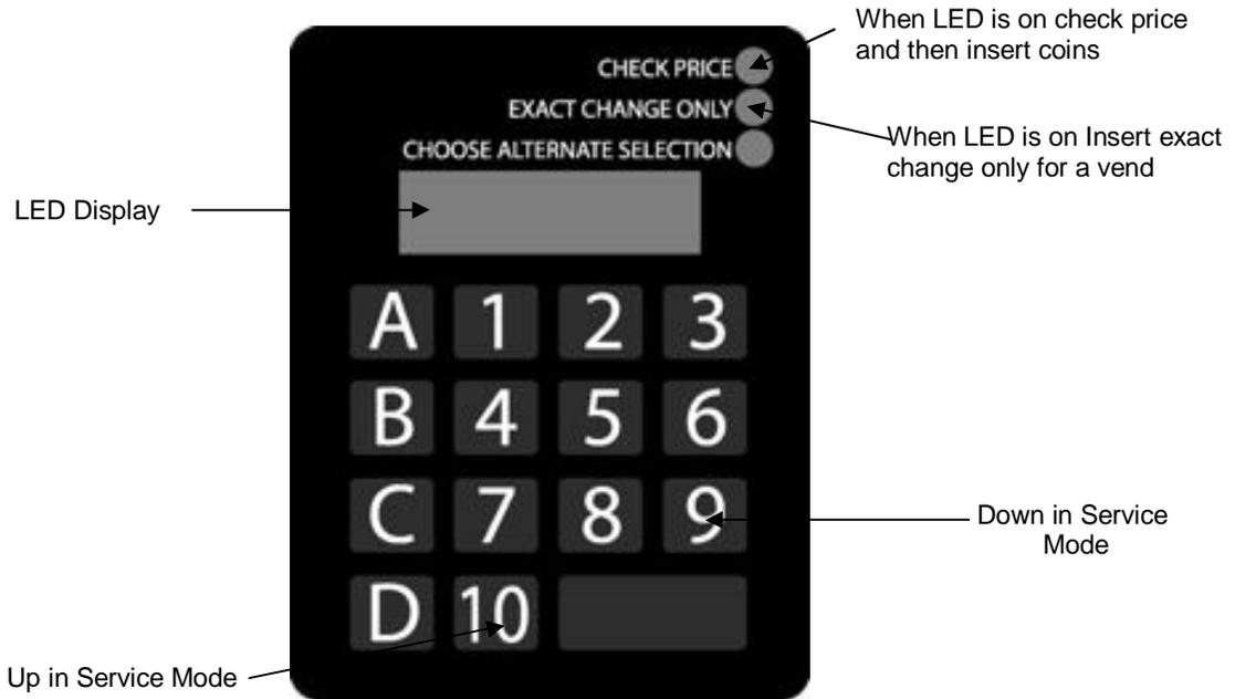
The LED Display shows the customer the amount of money entered into the vendor, and the cost of their selection, it shows the operator the Service Mode function for setting and testing the various functions of the vendor.
