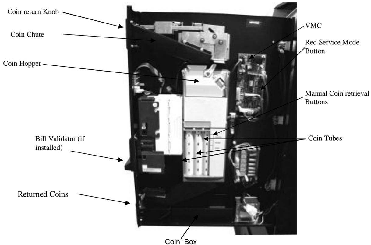
The Coin Return Knob pushes the Coin Return Lever, which returns inserted coins to the customer.
