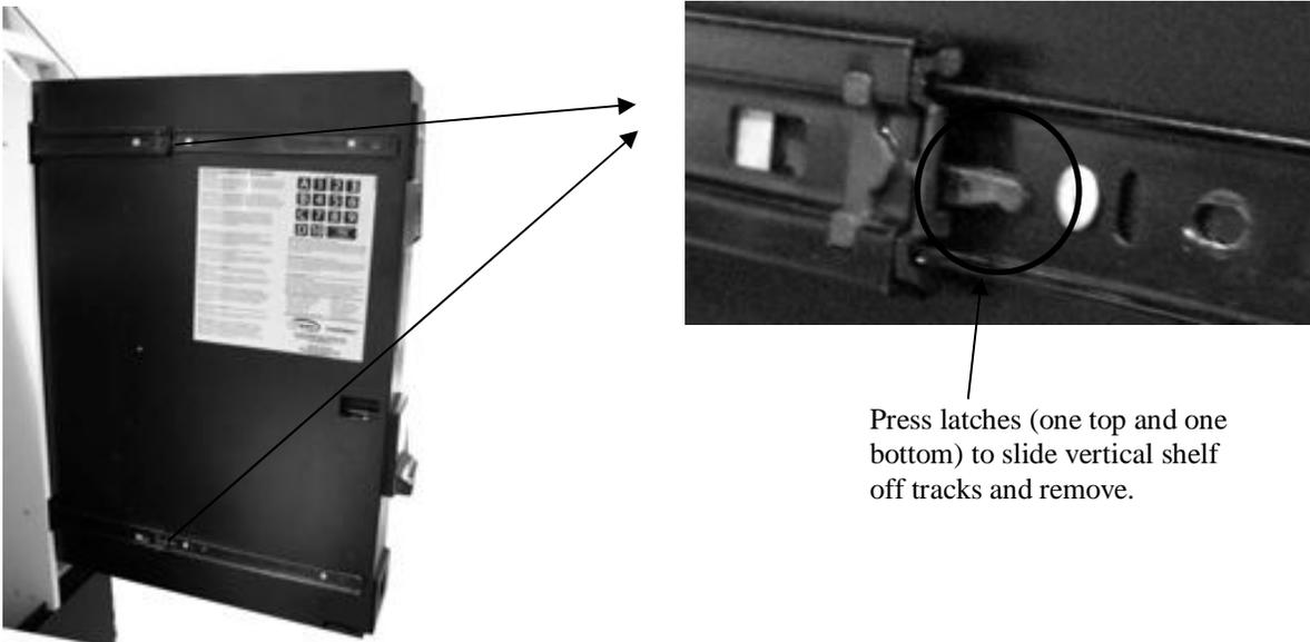
Press latches (one top and one bottom) to slide vertical shelf off tracks and remove.
