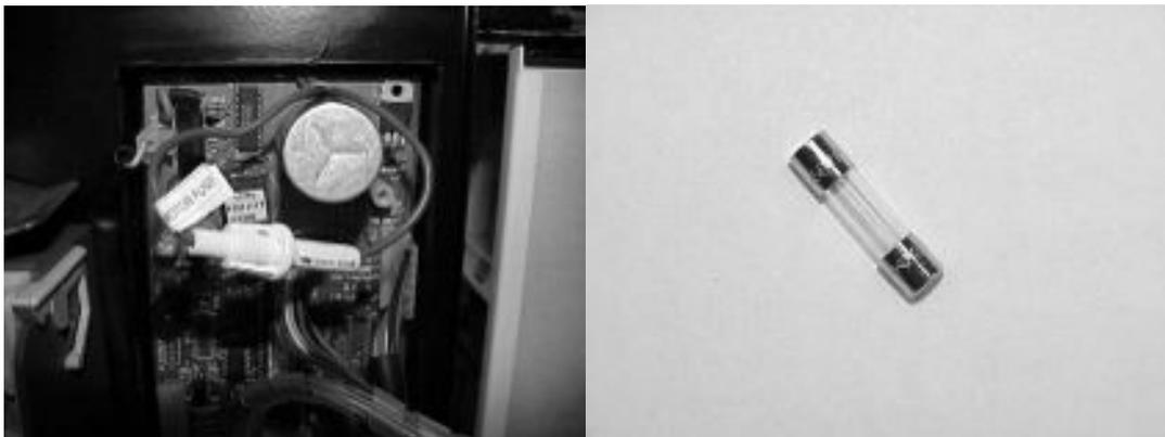
Shown above left is the EL243 VMC with fuse holder located on the vertical shelf. The motor fuse holder is labeled as such. The fuse in the above right photo is inside the holder and is a size 5x20mm and rated at 300 mA (0.300 amp) fast-acting.
