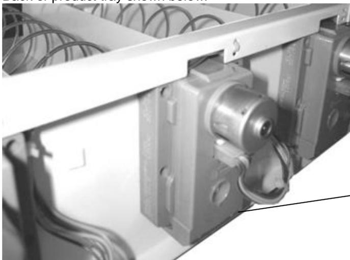
Motor is home when tab on shaft area lines up with arrow on motor housing
