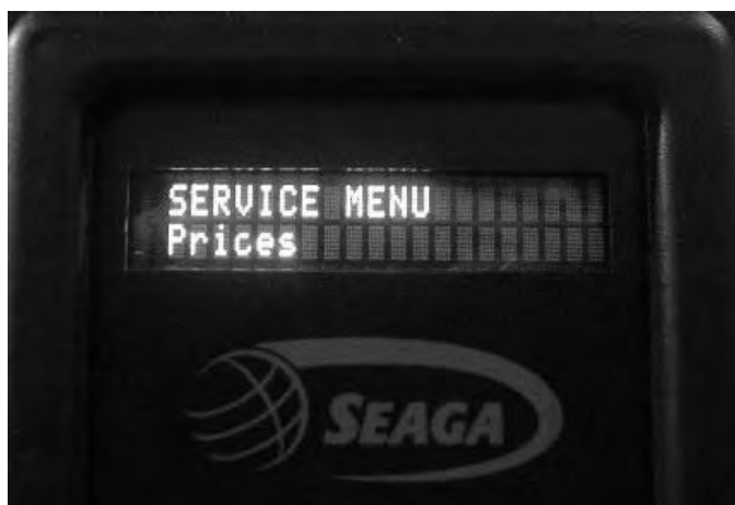
Fig. 11 – VFD Display while in Service Mode. The Prices menu is the first sub-menu.
